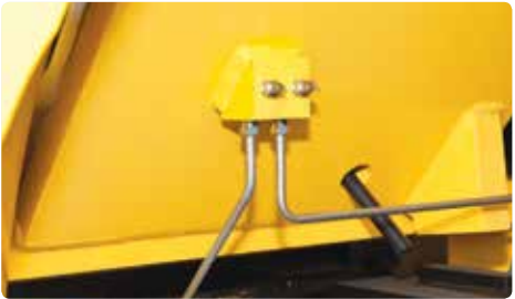
Greece inlet To facilitate the steering axle grease was applied remote type.
