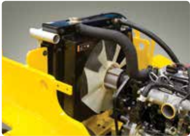
Aluminum radiator and coolers Aluminum radiator and coolers have been applied to increase the durability and heat output.
