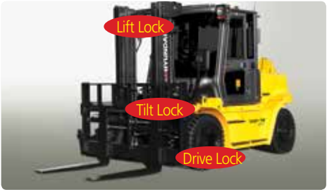
OPSS (Operator Presence Sensing System) Control of mast tilting, lifting and lowering is not possible through operation of the appropriate control when the operator is not in the seated position. (Option)
