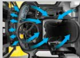
High-output air conditioner
