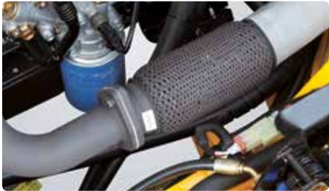
Expansion bellows The expansion bellows absorbs vibration and reduces noise generated from the exhaust gas system and also extends the life cycle of exhaust gas system.
