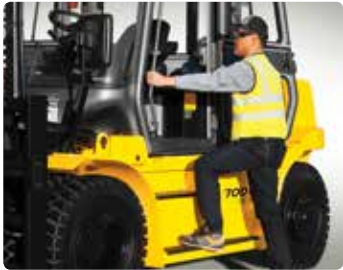
Large footboard & hand grip Wide“open”step offers convenience and safety when entering and exiting truck.
